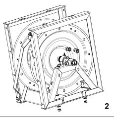
2) Bolt your hose reel to the ASSEMBLY FRAME/BRACE assembly. Use (4) M12 nuts and bolts and (8) M12 washers. Make sure the hose reel outlet (where the hose connects) faces away from the BRACE. A definition of the second sec
