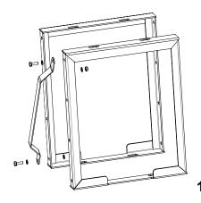
1) It's easiest if the BRACE is bolted to the ASSEMBLY FRAME first. This kit comes with 3 different sized braces for the 3 different length hose reels. The 150' hose reel uses the shortest brace, the 300' hose reel uses the average length brace and the 450' hose reel uses the longest brace. Do not fully tighten these bolts yet. Use (4) M8 nuts and bolts and (4) M8 washers. Be sure the cutout in the frame is on the bottom
